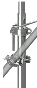
Swivel Coupler Reducer to connect a 48mm OD tube with the outer tube (60mm OD) of the prop for diagonal bracing.
