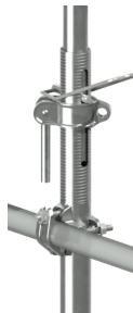
90° Right Angle Coupler Reducer to connect a 48mm OD tube with the outer tube (60mm OD) of the prop for horizontal bracing.
