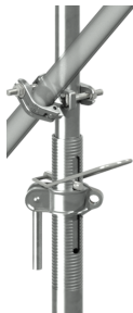
Swivel Coupler to connect a 48mm OD tube with the inner tube (48mm OD) of the prop for diagonal bracing.
