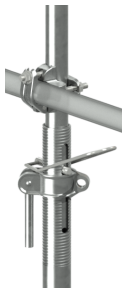
90° Right Angle Coupler to connect a 48mm OD tube with the inner tube (48mm OD) of the prop for horizontal bracing.
