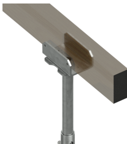
Single and Double U-heads provide extra support for bearers sitting on top of our Dynaton Acrow Props. To install on the prop, the stem of the U-heads slide inside the inner tube of the prop. Most type of bearers can fit within the single (W110mm x D200mm) or double (@200mm x D180mm) U-heads. Mainly for LVL bearers, our U-heads can also support many other beams as long as they can sit and fit properly on them. Dynaton also offers a wide range of LVL bearers . They have been tested for Australian/New Zealand Standards. Please contact us for availability.
